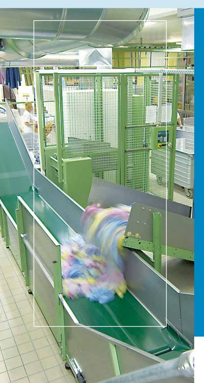
"Conveyor systems ensure reliable connections between the machines. We offer turnkey solutions for that."
